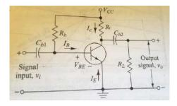
$$I_B = \frac{V_{CC} - V_{BE}}{R_b} = I_{B2} \approx \frac{V_{CC}}{R_b}$$
