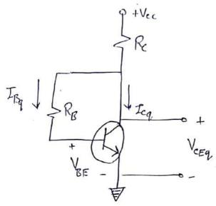
Applying KVL in Ball-emitter loop through Vec
