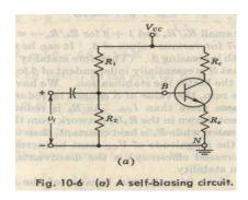
Solution The current in  $R_e$  is  $I_C + I_B \approx I_C$ . Hence, from the collector circuit of Fig. 10-6b, we have
